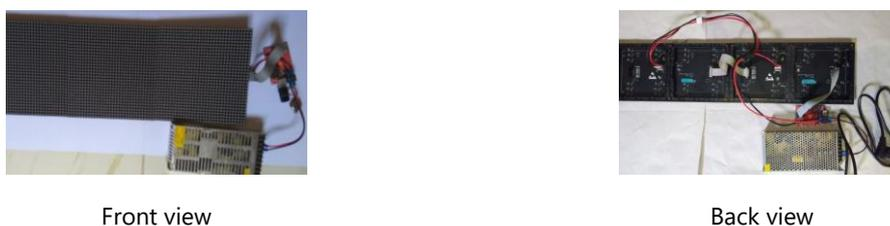
Figure 2. Series circuit of videotron panels
