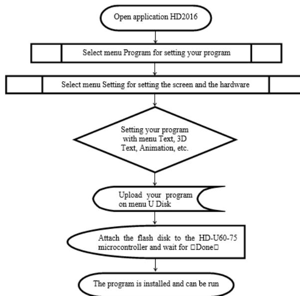
Figure 4. Flowchart of programming and installing videotron
