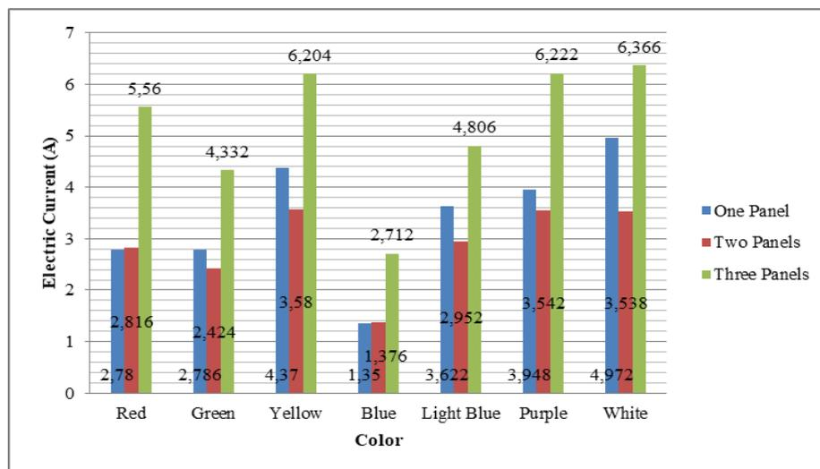
Figure 5. Data from the measurement of electric current in panel P.6 videotron with different background color
